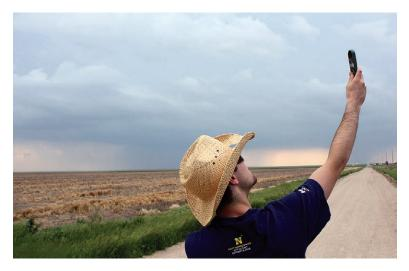
Fig. 2. Taking surface temperature and dewpoint temperature observations near Goodland, Kansas, on 23 May 2010 with a Kestrel 3500 ten minutes before tornado touchdown.
